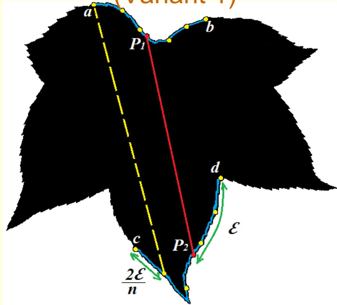
The red axis was obtained by skeleton method. Yellow points - two sets of equidistant points chosen according to  $p_1$  and  $p_2$  which belong to the skeleton axis and contour of the image. Yellow dashed - one of the test axes.
