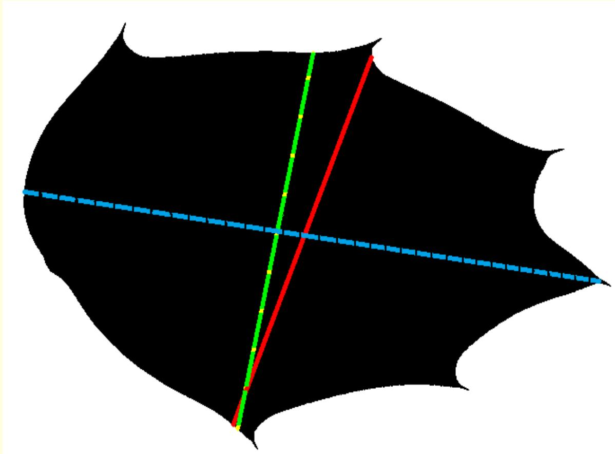
The example of image for which the symmetry axis obtained by skeleton method (red) and brute-force (green dashed line) significantly differ from the axis drawn by the expert (blue dotted line)
