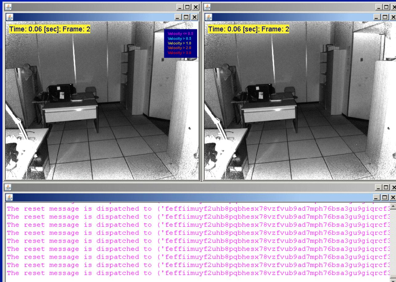
The **video data** to be transferred between the **agents** is **encapsulated** in built-in **class instances**. It is not necessary to encode huge video files using **Prolog** terms. The **data exchange** is based on **Java RMI**.
