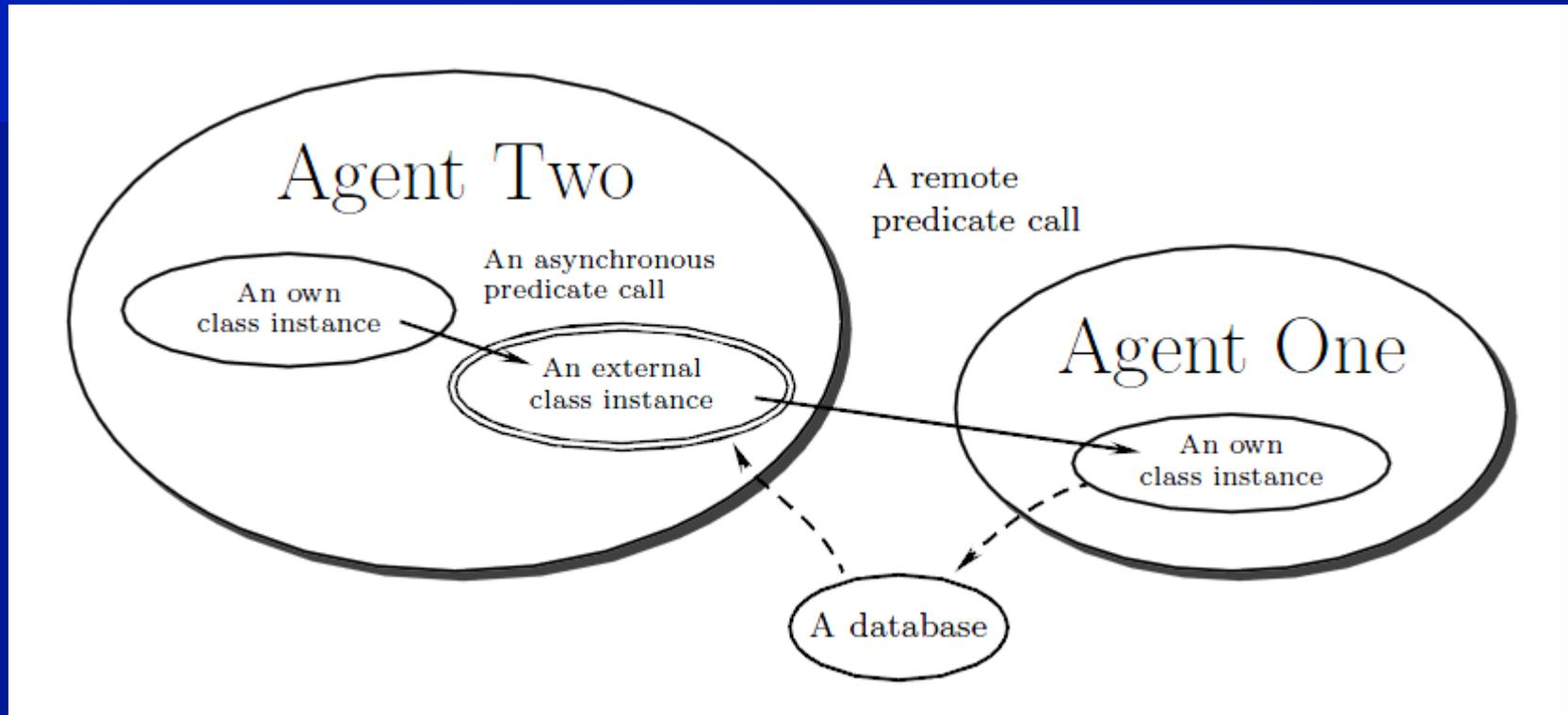
**Agent One** publishes an instance of a class in the external database. Then, **Agent Two** obtains this class instance and sends an asynchronous message to this class instance using **Java RMI**.
