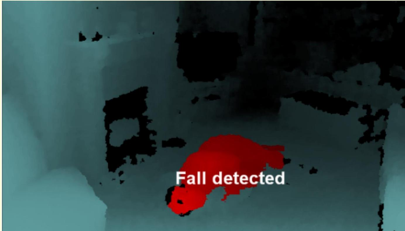
Simple cameras, environmental sensors, on-body sensors and depth cameras can be used in clients/patients behavior remote monitoring.
