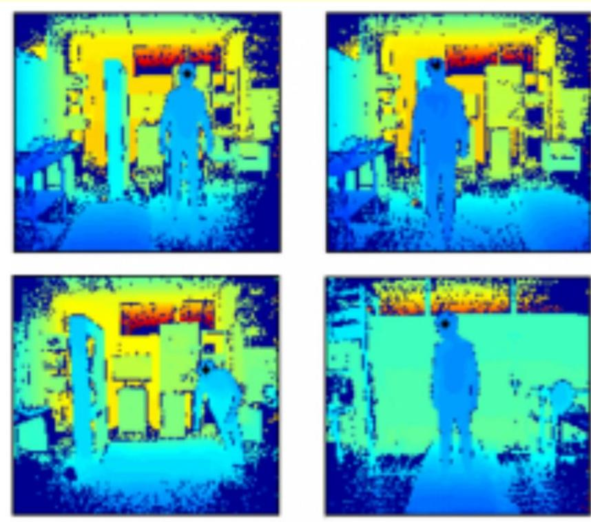
The dataset contains depth frames and skeleton joints collected using Microsoft Kinect v2 and acceleration samples provided by an IMU during the simulation of ADLs and falls.
